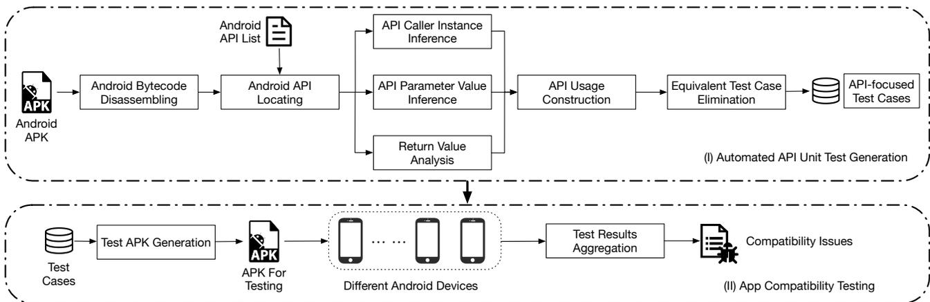
Figure 2: The working process of our approach.
